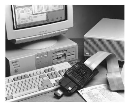
use real-time C debugger interface for the PC greatly simplifies the emulator command structure and allows even casual users to access the emulator's full potential. **HOST SYSTEMS SUPPORTED:** PC, SunSPARC, HP 700
